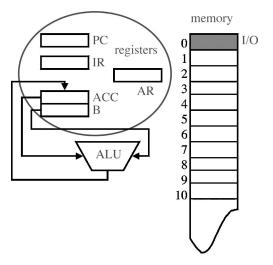
Fig. 1. One-Address Machine architecture.
