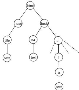
**Fig. 2.** An HTML page and the corresponding tag tree
