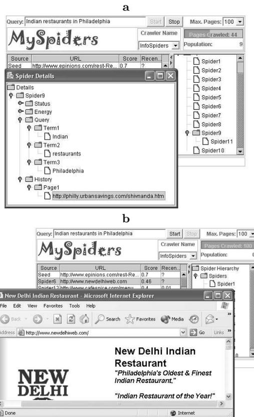
**Fig. 7.** The user interface of *MySpiders* during a crawl using the InfoSpiders algorithm. (a) In the search process; Spider 9 has reproduced and its progeny is visible in the expandable tree (right). A spider's details are revealed by clicking on it on the tree (left) (b) At the end of the crawl; one of the top hits is found by a spider (and it is not one of the seeds). The hit is viewed by clicking its URL in the results frame.
