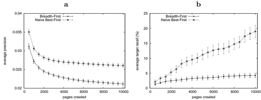
**Fig. 6.** Performance Plots: (a) average precision (similarity to topic description) (b) average target recall. The averages are calculated over 159 topics and the error bars show  $\pm 1$  standard error. One tailed t-test for the alternative hypothesis that the naive best-first crawler outperforms the breadth-first crawler (at 10,000 pages) generates  $p$  values that are  $< 0.01$  for both performance metrics.
