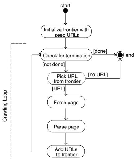
**Fig. 1.** Flow of a basic sequential crawler
