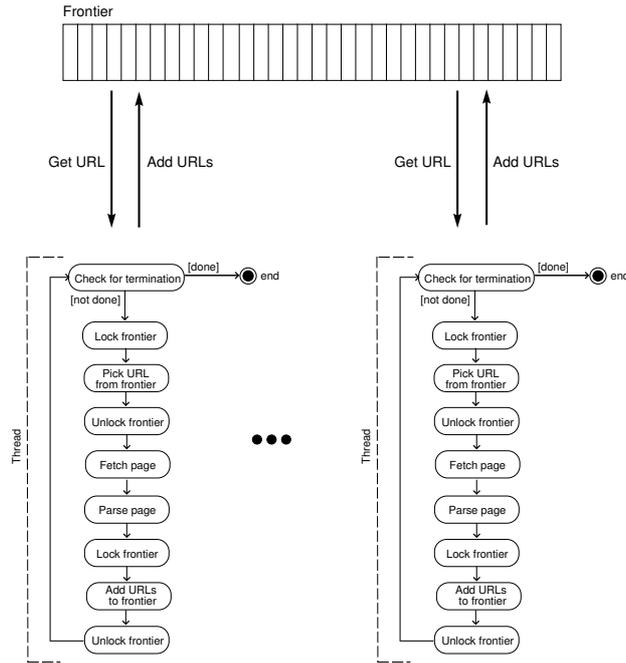
Fig. 3. A multi-threaded crawler model
